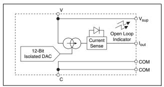
Figure 3. [c]FP-A0-200 Current Output Circuit
