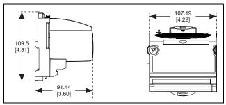
Figure 7. FP-AO-200 Mechanical Dimensions
