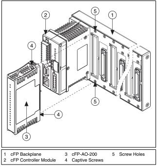
Figure 2. Installing the cFP-AO-200
