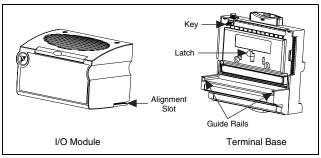
Figure 1. Installing the FP-AO-200
